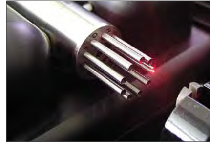
Laser Vision System infrared laser focused on a multi-tip punch
